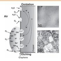
An effective method for nondestructive characterization of graphene defects is shown by enhancing oxidation of a Cu film underneath graphene through the graphene grain boundaries in air by electron injection supplied from electrochemical reaction of the graphene/Cu film. This process involves no appreciable oxidation of the graphene layer or the graphene grain boundary, as confirmed by detailed Raman and X-ray photoelectron spectroscopy.
