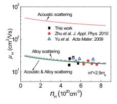
Alloy scattering dominated charge transport is found in the ZrNiSn thermoelectric solid solutions. A low deformation potential and a low alloy scattering potential are derived by a quantitative modeling of electrical transport properties, which is beneficial for a relatively high mobility. These intrinsic favorable features can contribute to the high power factors of the half-Heusler alloys.
