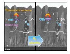
Enhanced mobility and conductivity are reached in polycrystalline zinc oxide films by hydrogen plasma post-deposition treatment. Optoelectrical characterization methods show that electron trap defects at grain boundaries are passivated, free electron concentration is increased, and that the electron transport is no longer limited by grain boundary scattering, even for non-intentionally doped films.
