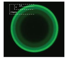
The inwards interweaving of polyamine and polyacid layers within an agarose matrix leads to the creation of well-defined, spherical multi-shells with different porosities. The higher the density of interweaving layers, the lower the porosity. The number and thickness of different levels of porosity are easily tuned by varying the number of polymer depositions and polymer concentration, respectively.
